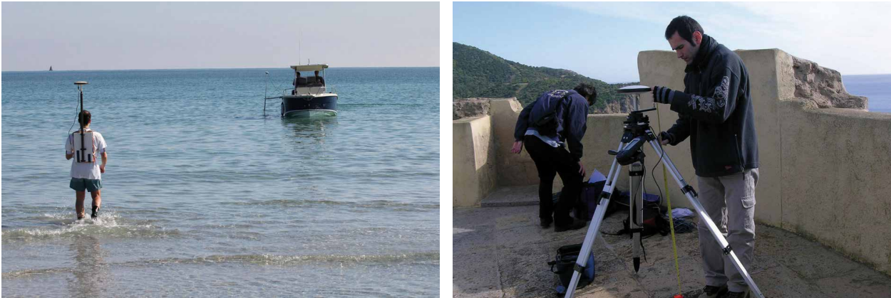
Figure 2. Production of the geodesic network, bathymetric sampling and study of marine currents.
